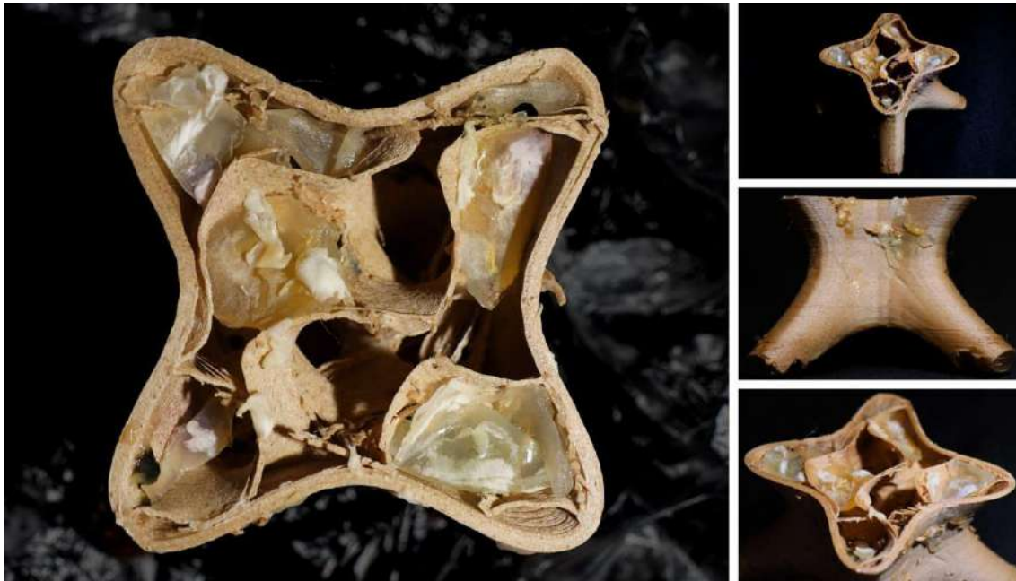
Figure 7. Living mycelium traces and details observed on the modules after inoculation.
