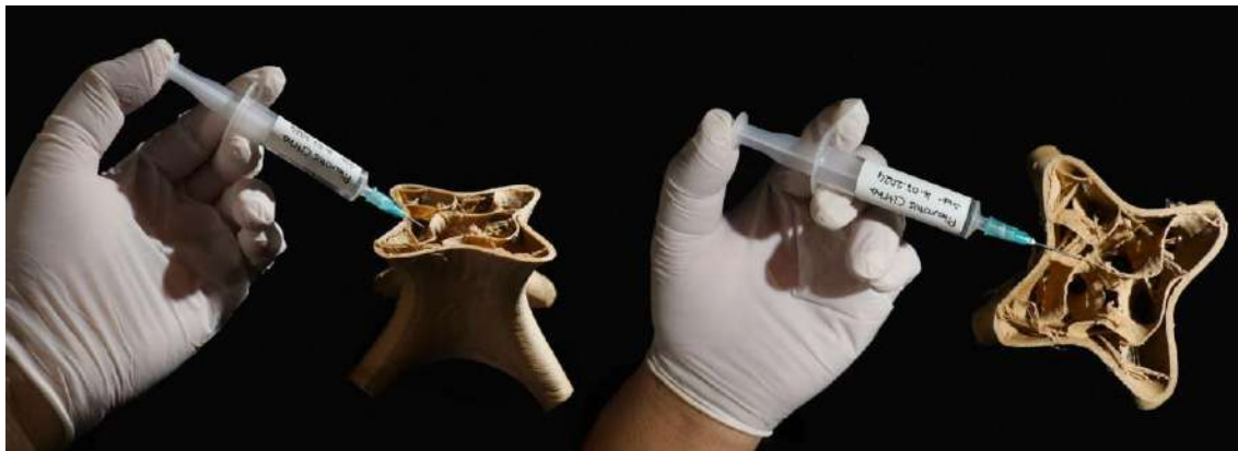
Figure 6. Inoculation of liquid mycelium into a module designed under controlled conditions, initiation of the mycelium cultivation process, and mycelium cultures on designed modules.
