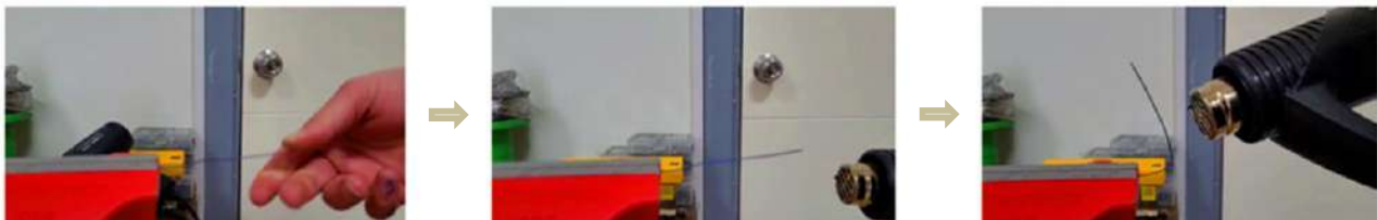
Figure 2. Test of straight wire memorized as a triangle (Photos by Hazel Almaç).
